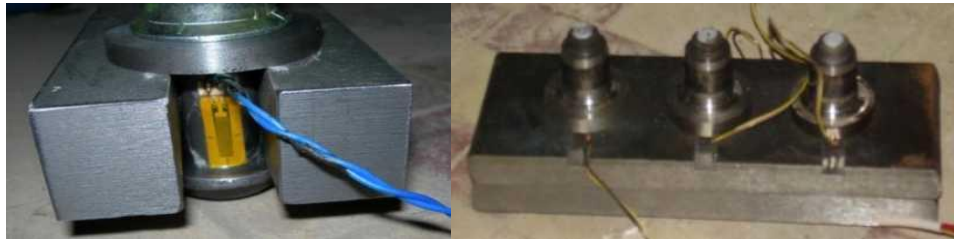
Fig. 10. Measurement of the tightness of the pin at the time of formation of the bar – connections
