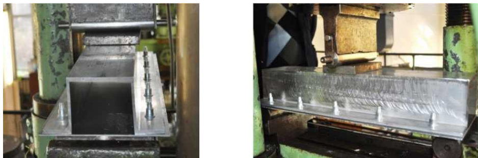
Fig. 3. General view of the 5th type specimen on supports of the testing machine TsDM-100
