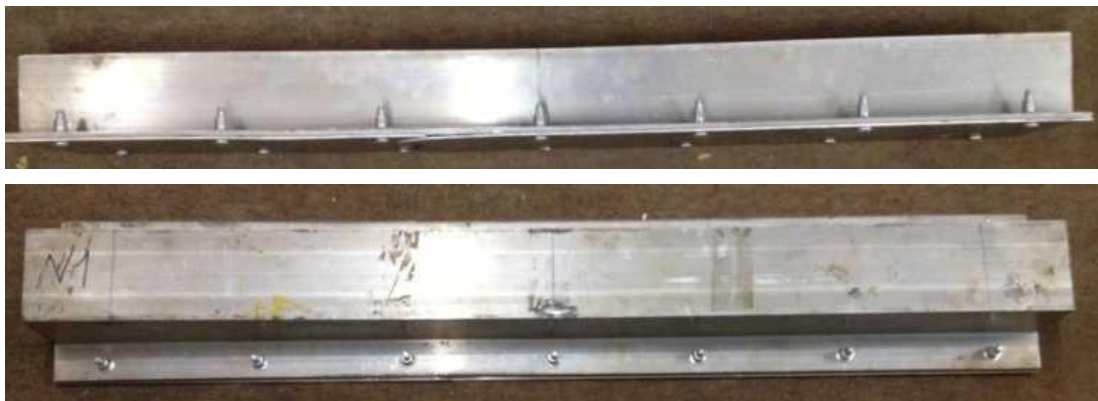
Fig. 6. General view of the sample with the PwCH connection of the type “BobTail”
